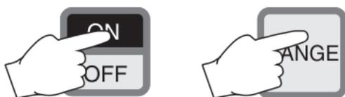
4. Make sure that the two additional decimal points are not displayed. If displayed, replace the battery before proceeding.
