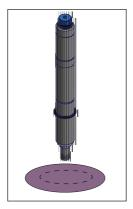
Gently rub the electrode tip of the slightly inclined probe over the paper.
