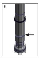
**6** Fill the trays through the opening. Screw the trays on the shaft until completely tightened.
