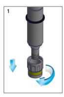
1 Keeping the probe in vertical position, unscrew membrane cap from the shaft.
