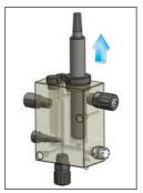
Uninstall the probe from PEF flow cell.
