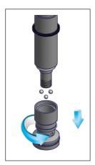
Unscrew the trays being careful to the 3 balls inside.
