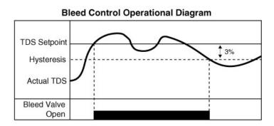
Hysteresis is just another name for "Deadband", which is the band between the two conductivity points at which the solenoid valve opens and at which it closes. The solenoid valve opens when the conductivity rises above the programmed setpoint and shuts when it drops to a level below the setpoint. This level is called Hysteresis and is a % of the setpoint.
