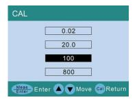
8) When cursor is on 100, put the calibration vial of 100 NTU into the sample well, close the cover and press (MEAS) to calibrate.
