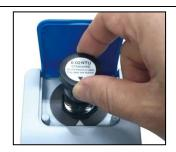
3) Open the flip cover and put in 0.02 NTU calibration vial. Align the arrow on the vial with the arrow on the sample well and then close the cover.
