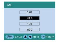
6) When cursor is on 20.0 NTU, put the calibration vial of 20.0 NTU into the sample well, close the cover and press MEAS to calibrate.
