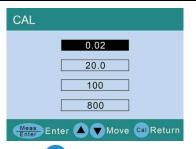
4) Press CAL key to enter calibration menu, and press MEAS key to perform calibration when cursor is on 0.02.
