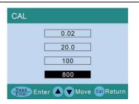
10) When cursor is on 800, put the calibration vial of 800 NTU into the sample well, close cover, and press key to calibrate.
