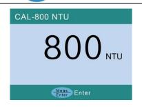
11) After calibration with 800 NTU standard, press MEAS key to confirm.
