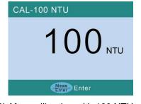
9) After calibration with 100 NTU standard, press MEAS key to return to calibration menu.
