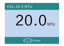
7) After calibration with 20.0 NTU standard, press ENTER key to return to calibration menu.
