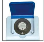
Apply small drop of silicone oil on the calibration vial and wipe even with soft cloth to improve light scattering. Please don't apply
