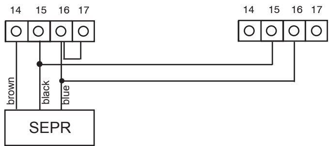
Configuration of a Flow Switch with a voltage free contact and two instruments
