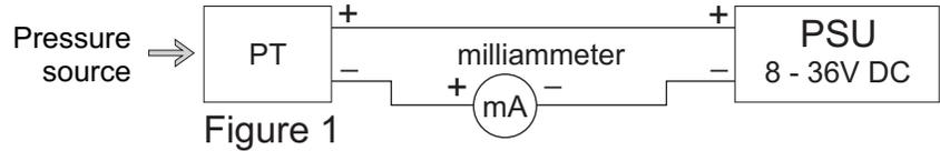
**Note:** Precision of calibration is determined by the accuracy of the pressure source and the accuracy of the milliammeter.
