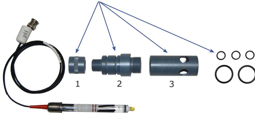
2. Slide two small O-rings over the Probe as shown below:
