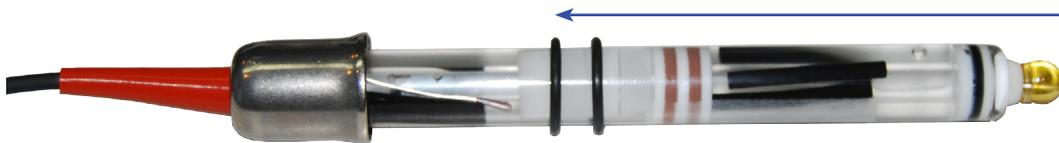
3. Slide the two small O-rings all the way up to the metal bell :
