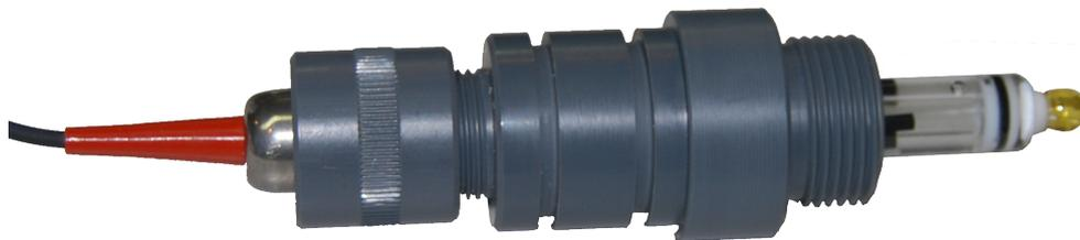
7. For Submersion mounting, slide the two large O-rings over the second connector into the slots indicated below :
