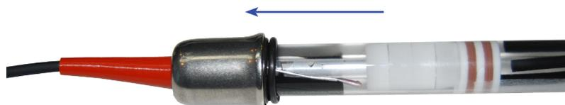
4. Slide the first connection over the BNC connector, as shown below, with the threaded end away from the cable. You will need to squeeze the white pH label around the BNC connector to get this into position.
