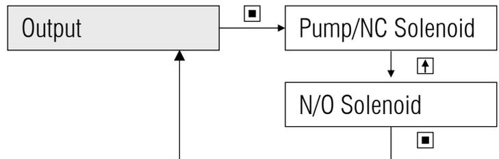
**Note:** Ensure that the output type is set correctly, as an incorrect setting can result in overdosing, or no dosing at all.
