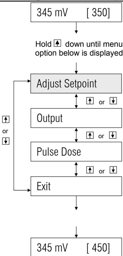
This is the desired ORP value of the process. To determine the setpoint, proceed as follows:
