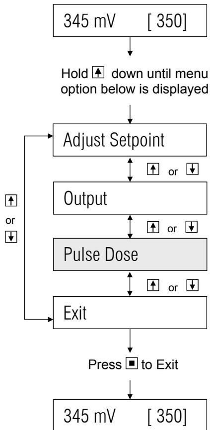
To leave the Pulse Dose/Duty Cycle in its default state, exit out of the menu. This is the factory default setting of ON/OFF=05s/90s which means that the pump will dose with this cycle setting when the system ORP is just below the mV Setpoint. Automatic adjustment of these times occurs when the mV level changes, explained below:
