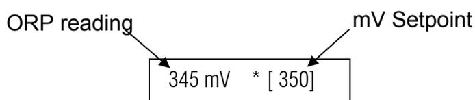
Display **during normal operation:** ORP of solution as reported by ORP probe as well as SETPOINT (shown between square brackets)
