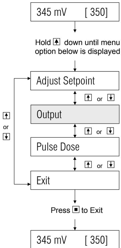
The MICRO-RX1 is a dosing controller, ie. the output activates a dosing pump or N/C solenoid, or de-activates a N/O solenoid, when the system ORP drops below the mV setpoint.
