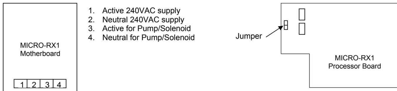
**NOTE:** The jumper indicated above should be removed or placed on only one of the 2 adjacent pins.
