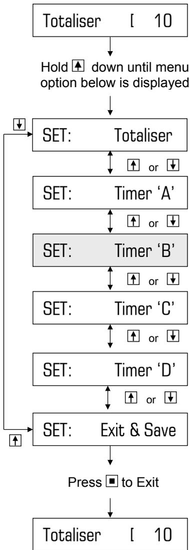
This is the time period when output/pump B will be active (i.e. ON).
