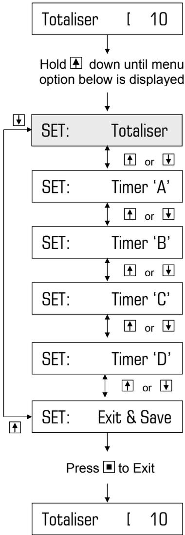
This is the pulse input number at which the outputs/pumps will be activated.
