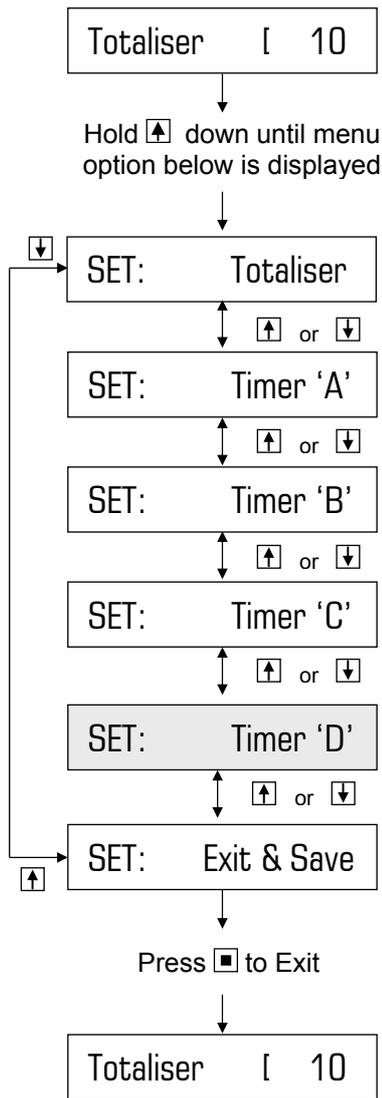
This is the time period when output/pump D will be active (i.e. ON).
