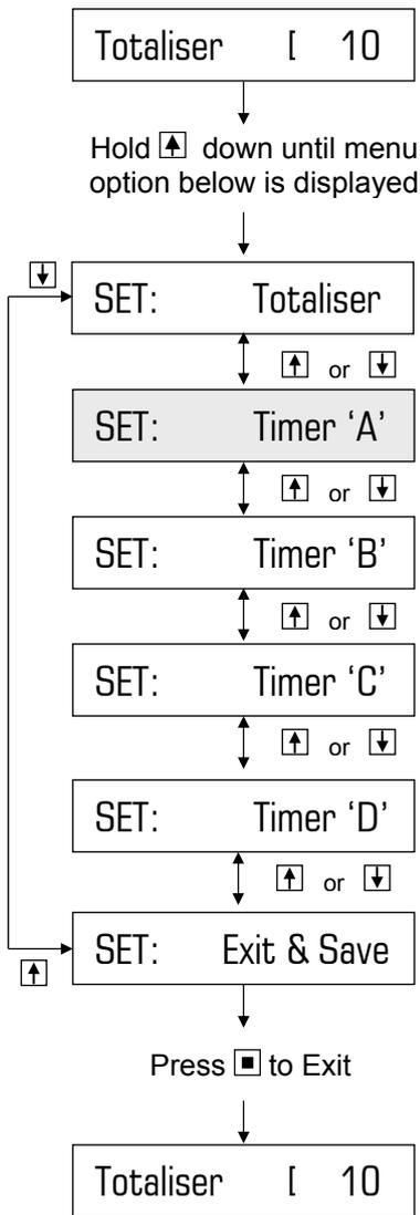
This is the time period when output/pump A will be active (i.e. ON).
