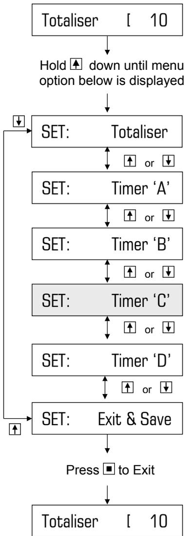
This is the time period when output/pump C will be active (i.e. ON).
