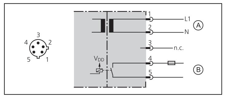
A: supply circuit B: output circuit
