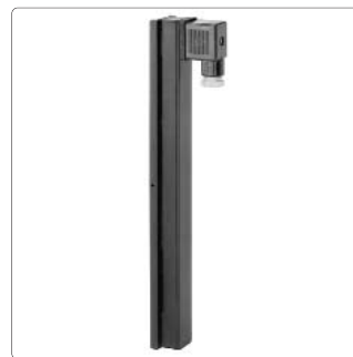
GEMÜ 1271 for DN 10, 15, 20 Instrument sensor for continuous flow readout (resistance 0-10 kΩ).
