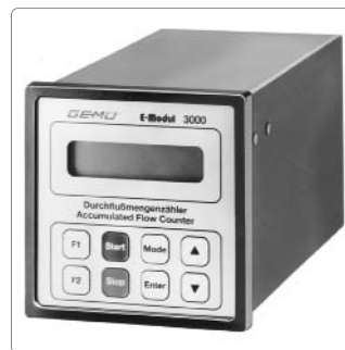
GEMÜ 3000 Accumulated flow counter with batch controller and signal transmitter (or transducer). Panel mounting acc. to DIN. 43700-96x96 Note: The mounting bracket is supplied with the unit as standard. (GEMÜ 3000 on the above photo is shown without mounting bracket.)
