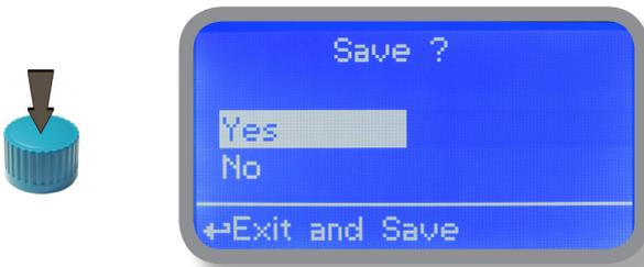
To end procedure move cursor on "OK" and press wheel to proceed to "Save" request screen. Move wheel on "YES" to save or "NO" to discard changes.
