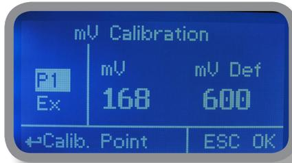
**Note:** This procedure assumes that instrument is correctly configured and a working ORP probe connected and installed on system. Measurement must be performed using plant water. Otherwise unattended results may occur.
