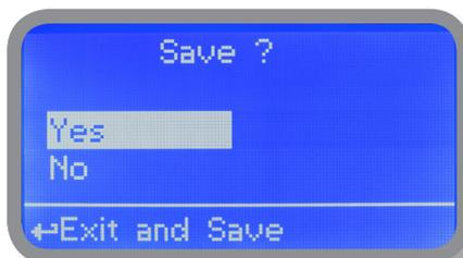
Choose "YES" to save changes. Exit from main menu. Main display will show a countdown including the selected peristaltic pump (left for pH peristaltic pump, right for ORP peristaltic pump). To stop this countdown go back to "Peristaltic pump activities" menu and choose "ON" as working mode or wait until countdown ends. **This function can be used for priming purposes.**
