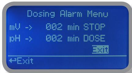
E.g. To set ORP peristaltic pump to stop after time ends and setpoint isn't still reached press wheel, choose maximum time, press wheel move on next field and choose "STOP". Time can be set between 0 and 100 minutes. When satisfied with settings move on exit and press wheel.
