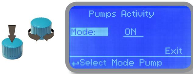
Move on "Mode" then press wheel. Choose "Man. Peristaltic pump1" for manually operate pH peristaltics pumps or "Man. Peristaltic pump2" for ORP peristaltic pump.
