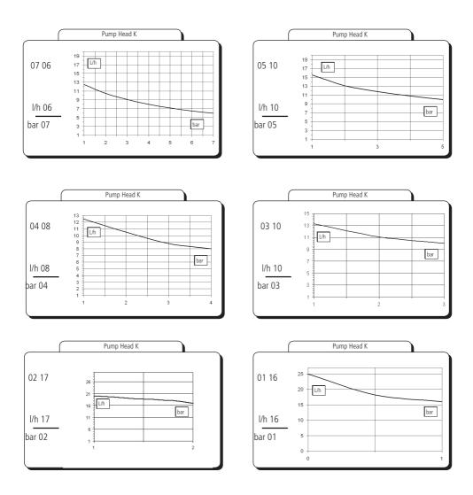
Flow rate indicated is for  $\rm H_2O$  at 20°C at the rated pressure.
