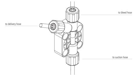
Self-venting pump head must be used when using chemicals that produce gas (i.e. hydrogen peroxide, ammonium, sodium hypoclorite at particular conditions).
