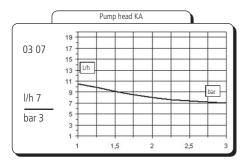
Flow rate indicated is for  $H_2O$  at 20°C at the rated pressure. Dosing accuracy  $\pm$  2% at constant pressure  $\pm$  0,5 bar.
