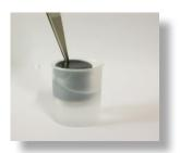
Cap(4) is located into a transparent box filled with storage solution. Pull out it(4) using a gripper and leave the storage solution into the box for future use.
