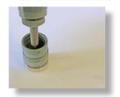
Put the sensor body(2) into the cap(4) filled with electrolyte.
