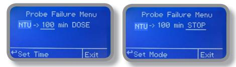
E.g. To set NTU pump to stop after time ends and probe doesn't change reading values press wheel, choose maximum time, press wheel move on next field and choose "STOP". Time can be set between 100 and 254 minutes. When satisfied with settings move on exit and press wheel.
