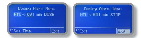
E.g. To set NTU pump to stop after time ends and setpoint isn't still reached press wheel, choose maximum time, press wheel move on next field and choose "STOP". Time can be set between 0 and 100 minutes. When satisfied with settings move on exit and press wheel.
