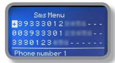
Up to three numbers for sending SMS can be stored into LDSTORBH memory. SMS recipient will receive an SMS containing instrument ID, NAME and status. Number formats can be stored using international prefix "+", international prefix "00" or local.
