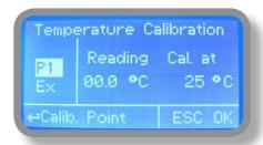
Note: This procedure assumes that instrument is correctly installed and configured, connected to a working NTC temperature probe (embedded). Calibrate using plant's temperature otherwise unattended results may occur.
