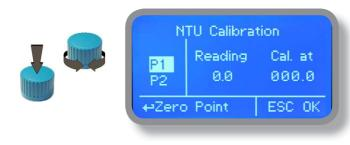
P1: zero value. Can't be edited. Dip probe's head into a ONTU solution and press wheel once reading field is stable.
