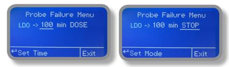
E.g. To set DO pump to stop after time ends and probe doesn't change reading values press wheel, choose maximum time, press wheel move on next field and choose "STOP". Time can be set between 100 and 254 minutes. When satisfied with settings move on exit and press wheel.
