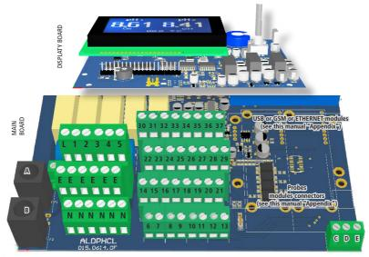
A: Main Fuse (6A T) B: Outputs Fuse (3.15AT) C - D - E: Factory reserved +5V
