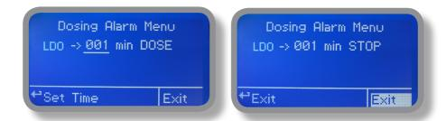
E.g. To set DO pump to stop after time ends and setpoint isn't still reached press wheel, choose maximum time, press wheel move on next field and choose "STOP". Time can be set between 0 and 100 minutes. When satisfied with settings move on exit and press wheel.
