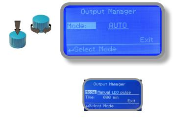
Press wheel to move cursor on "TIME" field. Once here, choose a working time between 0 (disabled) or 199 minutes. Move on "EXIT", then press wheel.
