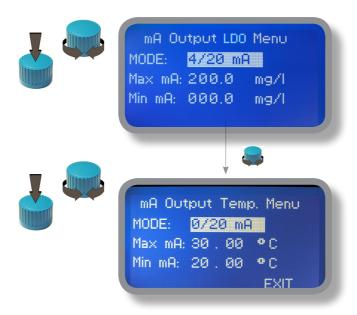
Rotate wheel to move within all 3 channels. Click wheel to selecte parameter and rotate wheel to change it. Click wheel again and rotate wheel to move cursor on next parameter. To end procedure move cursor on "EXIT" and press wheel to proceed to "Save" request screen. Move wheel on "YES" to save or "NO" to discard changes.
