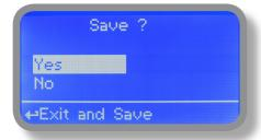
To end procedure move cursor on "OK" and press wheel to proceed to "Save" request screen. Move wheel on "YES" to save or "NO" to discard changes. If an error occurred during calibration procedure then the instrument will show an error message and will ask to proceed to a new calibration, cancel current operation or restore default settings.
