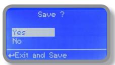
Choose "YES" to save changes. Exit from main menu. Main display will show a countdown for selected output. To stop this countdown go back to "Output Manager" menu and choose "AUTO" as working mode or wait until countdown ends. This function can be used for priming purposes.
