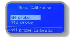
In the following example instrument will calibrate pH using default buffer solutions values.
