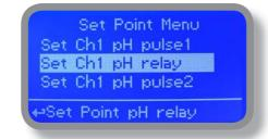
Proportional mode set the instrument to operate using a calculated percentage between two set values that enable or disable the pH pump. To use this mode move cursor on "Working Mode". Press the wheel and select it.
