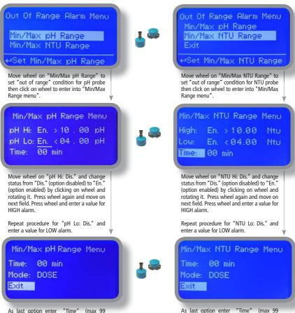
As last option enter "Time" (max 99 minutes) after which if lower or higher read value condition stays then the alarm occurs (to set into mode field).
