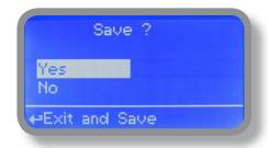
To end procedure move cursor on "OK" and press wheel to proceed to "Save" request screen. Move wheel on "YES" to save or "NO" to discard changes.
