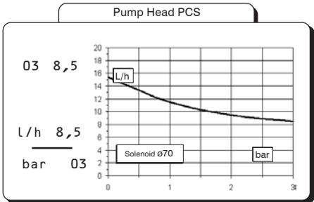
Flow rate indicated is for H<sub>2</sub>O at 20 °C at the rated pressure. Dosing accuracy ± 5% at constant pressure ± 0,5 bar.
