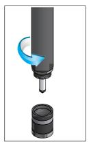
Move down the o-ring (rubber band) in order to allow bleed air from the underneath micro-hole.
