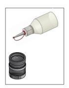
Fill up completely the membrane cap with the electrolyte gel.
