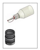
Fill up completely the membrane cap with the electrolyte gel.
