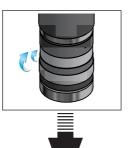
Move up the o-ring (rubber band) to its seat and move second oring over the first to obtain only one ring.
