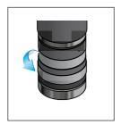
Move down the o-ring (rubber band) in order to allow bleed air from the underneath micro-hole...
