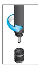
Unscrew membrane cap and discard the remaining electrolyte.
