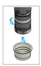
Move down the o-ring (rubber band) in order to allow bleed air from the underneath micro-hole and remove the transparent cover.
