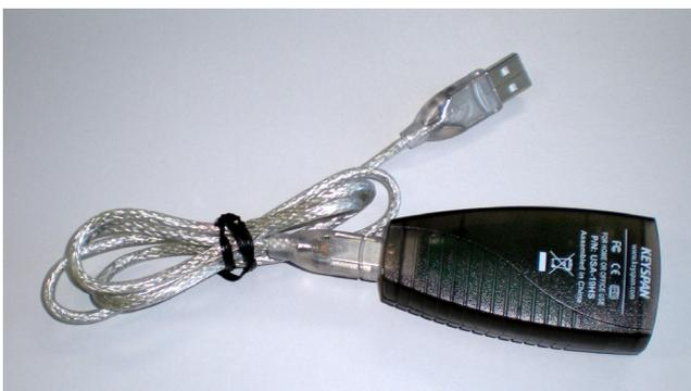
For computers that only have USB ports, and not a serial port; Use this adapter to connect the Serial data download cable to the USB port.
