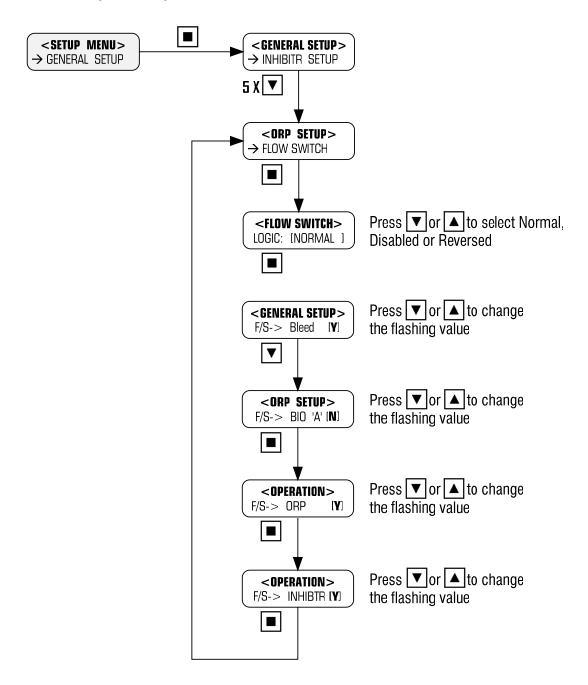
None, one, two, three or all four of the outputs can be selected to be disabled if there is no flow. Typically, the Bleed, ORP and Inhibitor outputs are disabled if there is no flow and the Biocide 'A' doses during its program regardless of the flow status. However the Biocide 'A' output can be set to be disabled if there is no flow.
