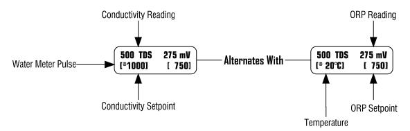
**NOTE:** An asterisk '\*' flashes on the screen when the controller receives a pulse from an optional water meter.
