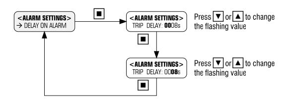
When an alarm condition is detected, eg High Conductivity or ORP Alarm, the relay only trips immediately if the Trip Delay is set to 0 seconds. However, if alarms do not become immediately critical, it is better to program a delay on the alarm to prevent "nuisance trips".
