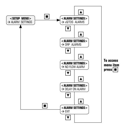
The controller has 5 programmable alarm functions as outlined above. If any of the alarms are activated and confirmed, the common alarm contact switches, the red Alarm LED illuminates, and the Alarm message is displayed on the LCD.
