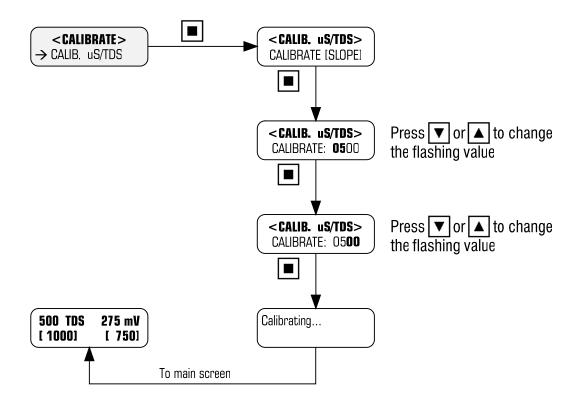
The zero is factory set so should not require calibration. However, if the display reads above zero with the conductivity probe disconnected, recalibrate the zero as follows:
