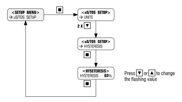
Hysteresis is the deadband between the two conductivity points at which the solenoid valve opens and closes. The solenoid valve opens when the conductivity rises above the programmed setpoint and shuts when it drops to a level below the setpoint. This level is called Hysteresis and is a % of the setpoint.
