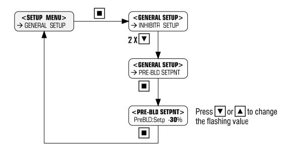
In the example above, the Pre-Bleed setpoint is set as the Normal Conductivity Setpoint less 10%. Hence, during the Pre-bleed time (ie. Immediately before biocide dosing), the normal conductivity setpoint is reduced by 10%, and the controller will try to maintain this reduced setpoint until biocide dosing commences. The objective of pre-bleed is to allow for a longer Bleed Lock-out duration without the risk of entering scaling conditions.
