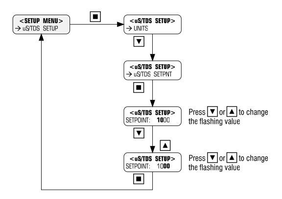
The Bleed Setpoint is the desired conductivity value of the process (displayed in TDS or  $\mu$ S). When a solenoid valve is connected to the bleed output, the valve opens when the conductivity rises above the setpoint. When this occurs, the tower water is flushed to drain and fresh make-up water dilutes the system, thus lowering the conductivity of the tower water. The valve shuts when the conductivity drops to the hysteresis value (explained in the next section). The cycle repeats.
