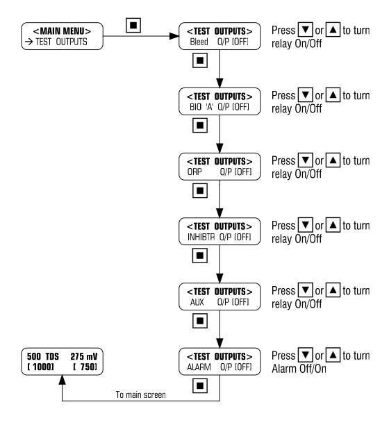
When any of the Outputs is activated, the respective Output LED illuminates and the Output relay switches, putting 240VAC power onto the output terminal, which activates the pump or solenoid valve wired to it.
