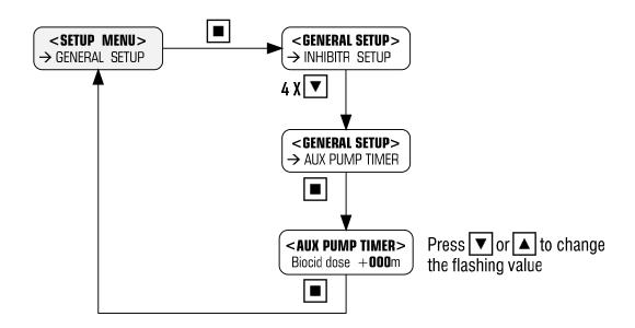
Often when biocides are dosed into the manifold of the DIGICHEM-ORP-XP2 systems, the circulating/ condenser pump of the cooling tower is not running. This can cause problems of clogging and corrosion in the manifold, as well as biocide not being dosed into the cooling tower water.
