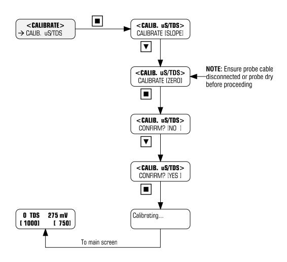
If you inadvertently calibrate the zero and/or slope to the incorrect values, and you cannot recover by repeating the normal calibration procedure, then you can reset the calibration and start again.
