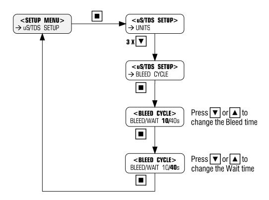
In the example above, the solenoid bleeds 10 seconds during every 50 second cycle (ie 10+40), which equates to a 20% bleed cycle.
