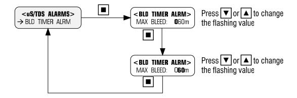
The Bld (Bleed) Timer Alarm is the maximum acceptable bleed time for the system to reach the Setpoint. This alarm is designed to protect the system from excessive bleeding in the event of a false reading from a faulty Conductivity probe, or if the controller itself is faulty.
