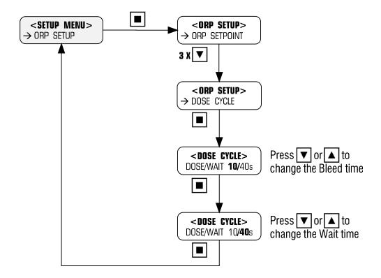
In the example above, the pump doses 10 seconds during every 50 second cycle (ie 10+40), which equates to a 20% duty cycle.
