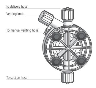
Flow direction is indicated by the arrow on the valves.
