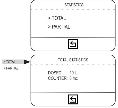
DOSED: total quantity dosed (max 999.999.999 L). COUNTER: water meter counter (cubic meter of water).
