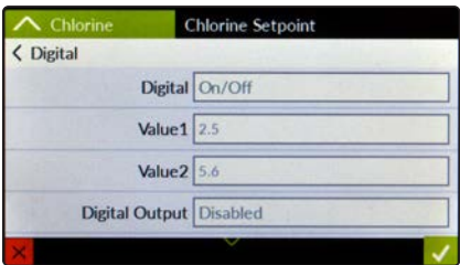
Digital Setpoint configuration sample having two values to work on.
