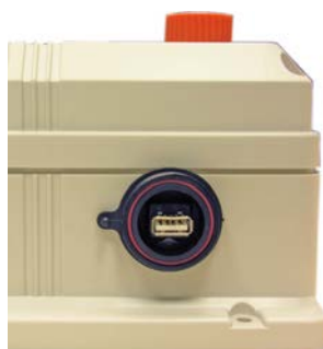
Insert USB pendrive here (right side of instrument) After usage put back USB cap
