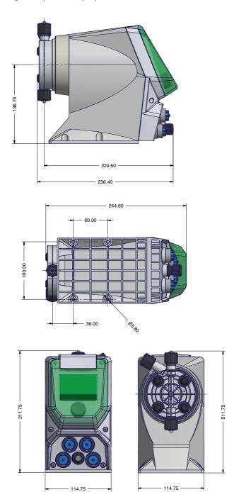
Fig. 3. Pump dimension - pump head mod. N
