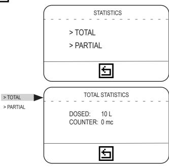
DOSED: total quantity dosed (max 999.999.999 L). COUNTER: water meter counter (cubic meter of water).
