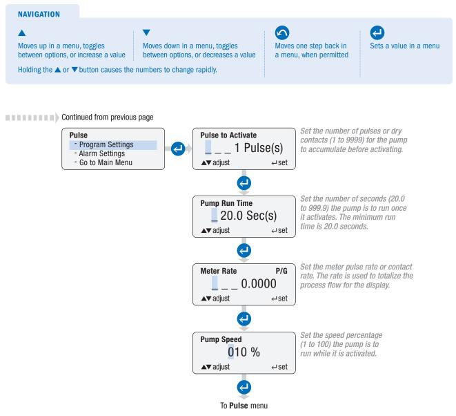
After settings are entered the display returns to the **Pulse** menu and **Alarm Settings** can be programmed.
