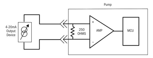
Pump signal impedance is 250 ohms.
