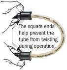
Place the new tube in the pump head.
