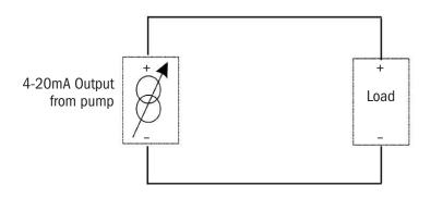
The pump sources the voltage for the output signal loop at 24VDC. The pump will control the magnitude of current on the loop (from 4 to 20mA) according to the speed that the pump is running at. The maximum loop impedance (load on the output signal loop) is 300 ohms, which includes the load plus any resistance due wire length, connections, etc.
