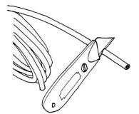
Cut off the calcified or blocked section.
