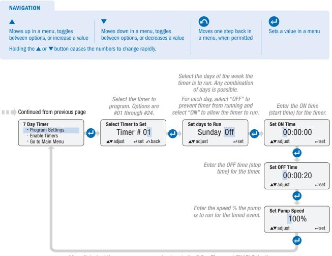
After all desired timers are programmed, return to the 7 Day Timer and ENABLE the timers.
