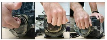
Hold the motor securely with one hand. With the other hand, hold the tube housing cover with your forefingers inside the top lip of the cover. Use the cover as a wrench and with your palm quickly (snap) rotate the cover counterclockwise to collapse the roller assembly. The tube will no longer be pressed against the tube housing wall.
