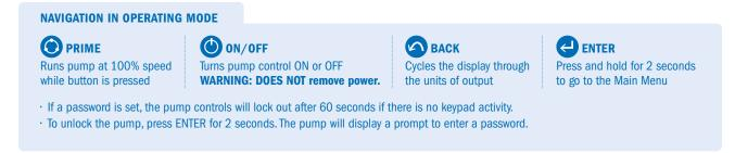
This example shows the MANUAL operating display. The password steps are the same from any operating display.
