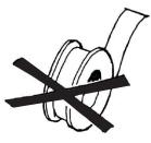
DO NOT use thread seal tape on pump tube threads.
