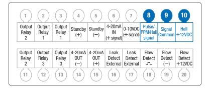
▲ **CAUTION** The 12VDC supply from connection #10 is limited to 20mA and is only for powering Hall Effect sensors on turbine or paddlewheel type flow meters. Do not use the 12VDC output for anything else; otherwise, damage to the pump will occur.
