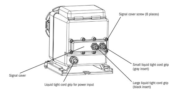
**CAUTION** Signal cables must be UL, cUL AWM Style 2464 approved with conductors between 28 AWG and 18 AWG. Jacket diameter for small liquid tight must be 0.064" to 0.210". Jacket diameter for large liquid tight must be 0.114" to 0.250".
