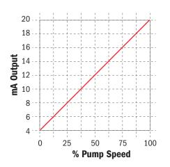
This signal corresponds proportionally to pump speed with 0% pump speed equaling 4.0mA and 100% pump speed equaling 20.0mA. The signal response is not adjustable by the user.
