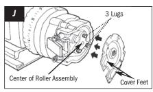
Align cover feet near the bottom
