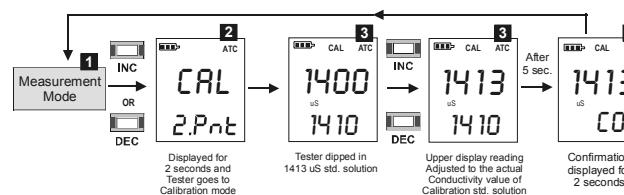
Figure 8: One-point manual calibration sequence for EC Testr11+
