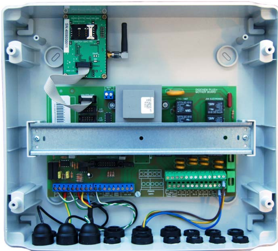
DIGICHEM Plus+ MOTHER BOARD WITH GSM/3G MODEM CARD INSTALLED
