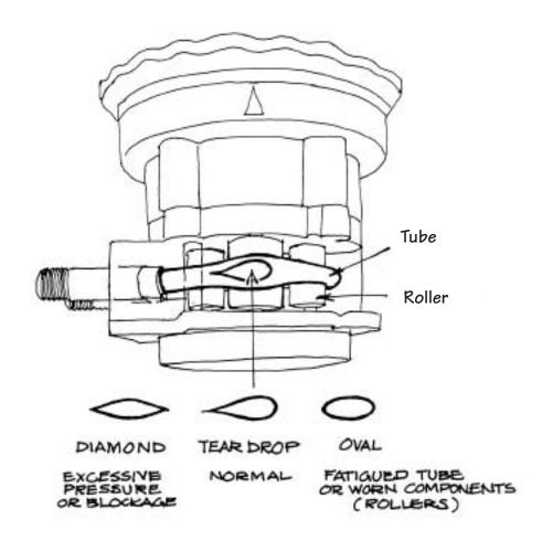
The tube can rupture or break. A rupture normally occurs at the point between the discharge tube fitting and the area where the roller leaves the tube. A break or rip occurs just past the suction fitting. The tube is the workhorse of the pump. It is perishable and eventually has to be changed.
