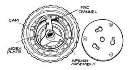
The feed rate control adjusts the output by utilizing a cam and lifter system to control the rotation of the roller assembly according to the setting on the dial ring.
