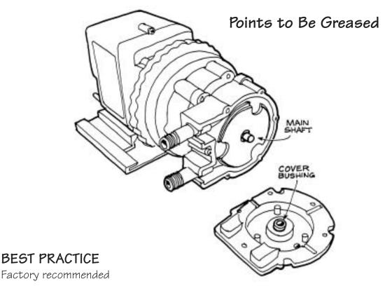
Every time pump is serviced or a tube is replaced, apply grease (AquaShield®) to the pump head cover bushing and main shaft ONLY.
