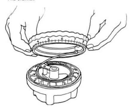
**14.** To secure mounting plate, align its arrow with the FRC housing arrow and install the three screws.
