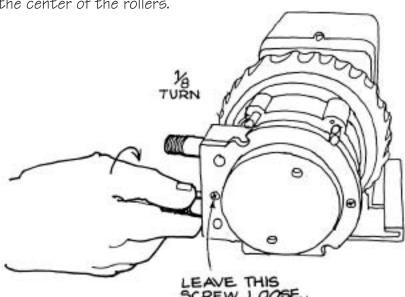
**4.** Turn the pump off, let go of fitting, and tighten the cover screws. The cover is not on securely if there is a gap between the screw boss and the cover.
