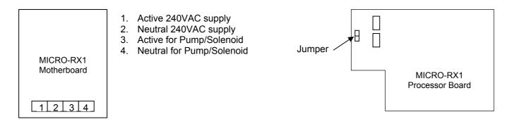
**NOTE:** The jumper indicated above should be removed or placed on only one of the 2 adjacent pins. The BNC connection for the ORP electrode and the connection for the Earth Probe are situated on the outside of the enclosure at the bottom left hand side.
