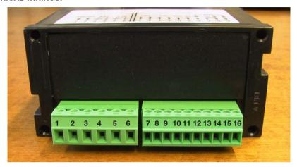
1 - 2: Power Supply (24VAC\* or 115VAC\* or 230VAC\*). \* See instrument's label
