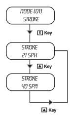
Choose "stroke" working mode: "SPH" (strokes per hour) or "SPM" (strokes per minute) .
