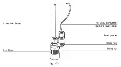
Connect BNC from level probe into pump's level input (front side of the pump). Put level probe assembled with foot filter into tank's bottom.
