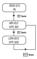
To work in this mode is necessary to specify the "HImA" (maximum working current), "LOmA" (minimum working current) and "SPM" (strokes per minute) values that pump will produce between the parameters.
