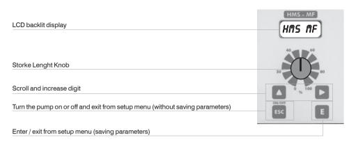
The "HMS MF" pump is equipped with a keyboard. To avoid any misunderstanding during next chapters all keys will be described as shown on this legend:
