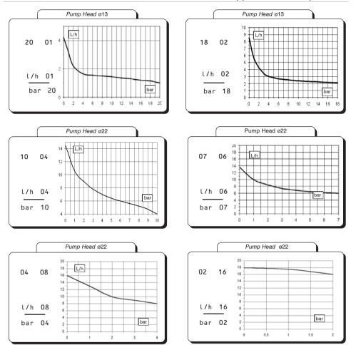
Flow rate indicated is for  $H_2O$  at  $20^{\circ}C$  at the rated pressure. Dosing accuracy  $\pm$  2% at constant pressure  $\pm$  0,5 bar.
