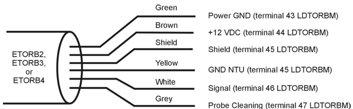
Note that the Signal Ground (yellow) and Power Common (green) conductors and the probe's stainless steel case are electrically connected together within the probe.
