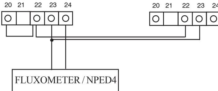
If the flow sensor with free of voltage contact Normally Open when there is flow, set “Flow” on “reverse” in the “Option” menu.
