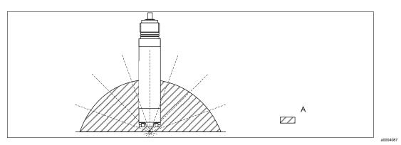
Fig. 3: Angle of installation
