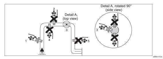
Fig. 13: Permissible and impermissible sensor installation positions
