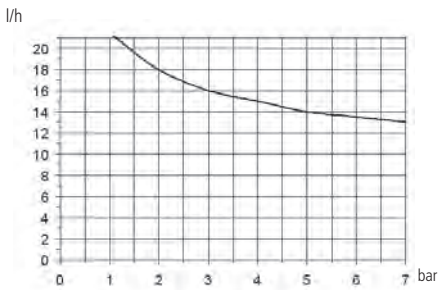
0713: l/h 13 bar 7 Pump head mod. NA
