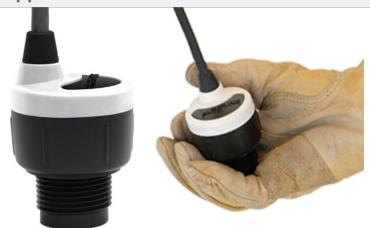
The general purpose ultrasonic level transmitter provides continuous level measurement up to 49.2" (1.25m) with a 4-20 mA signal output, and is configured via our free WebCal software. This non-contact liquid level sensor is ideally suited for corrosive, sticky or dirty liquids, and is broadly selected for small day tank, skid, IBC, sump and process tank level applications.
