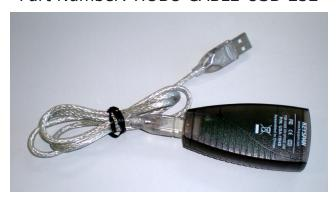
For computers that only have USB ports, and not a serial port; Use this adapter to connect the Serial data download cable to the USB port.
