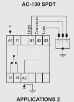
Connection of three probes (CP-3C) for DC applications.
