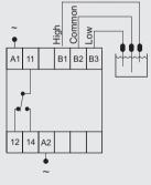
APPLICATION 1 Connection of three probes (CP-3C)
